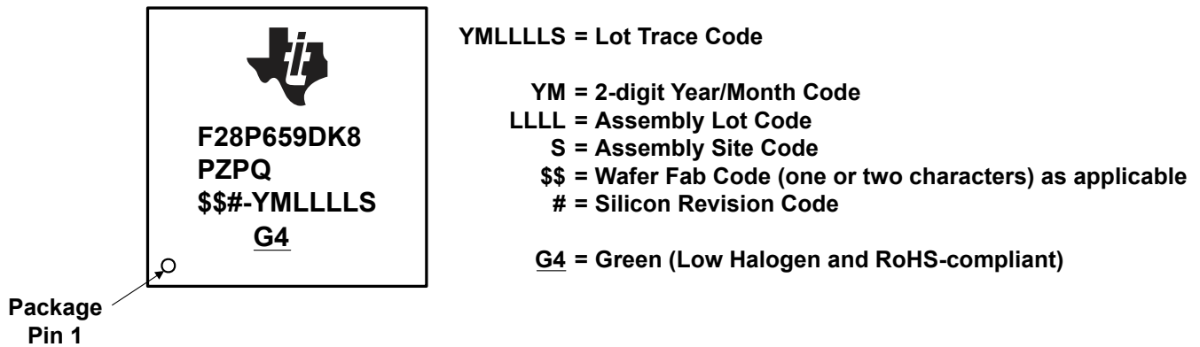
Figure 9-8. Package Symbolization for PZP Package – Automotive
