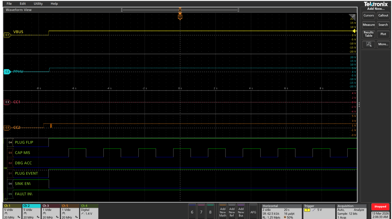
Figure 9-1. PD Contract with Capability Mismatch and PPHV Enabled
