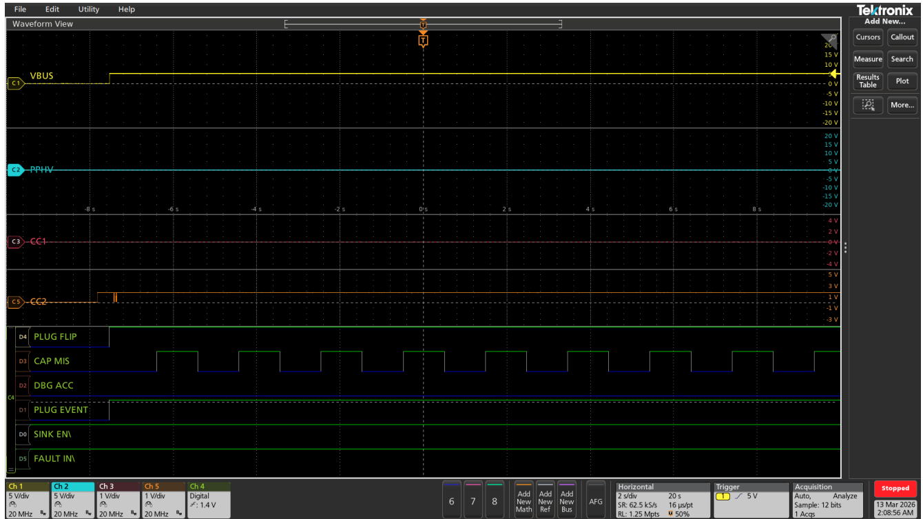
Figure 9-2. PD Contract with Capability Mismatch and PPHV Disabled
