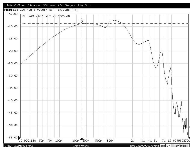
Figure 8-24. Off-state Data-Switch Isolation vs Frequency
