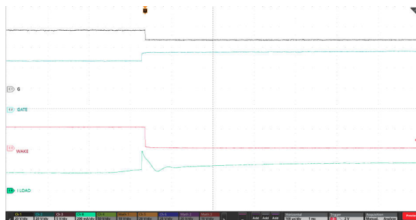
Figure 9-4. Zoom-In View of State Transition From LPM to Active Mode ( \overline{\text{LPM}} = Low, V_{\text{IN}} = 48V, \text{EN}/\text{UVLO} = High)
