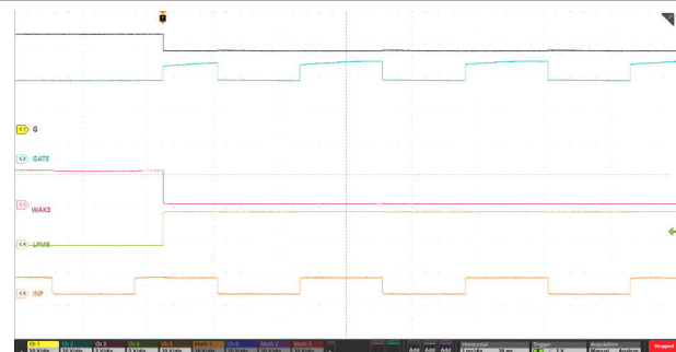
Figure 9-7. With \overline{\text{LPM}} = Low to High, \text{INP} Gained Control on GATE ( V_{\text{IN}} = 48V, No Load)
