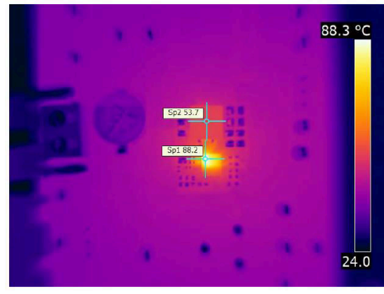
Figure 6-14. Thermal Image at 14-A Output Current
