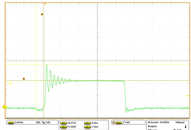
Figure 6-22. Switch Node Ringing and Dead-Time at 10-A Output Current
