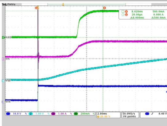
Ch1: Input voltage; Ch2: Soft-start (SS) voltage; Ch3: Input current; Ch4: LED current; Time: 2 ms/div
