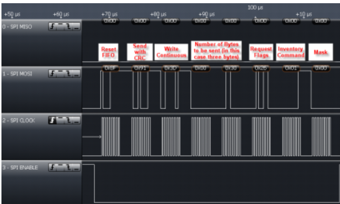
Figure 6-22. Inventory Command Sent From MCU to TRF7964A
