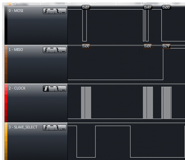
Figure 6-26. Reset FIFO and Read RSSI
