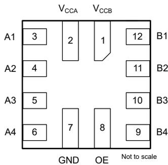
**Figure 4-3. RWB Package, 12-Pin X2QFN (Top View)**
