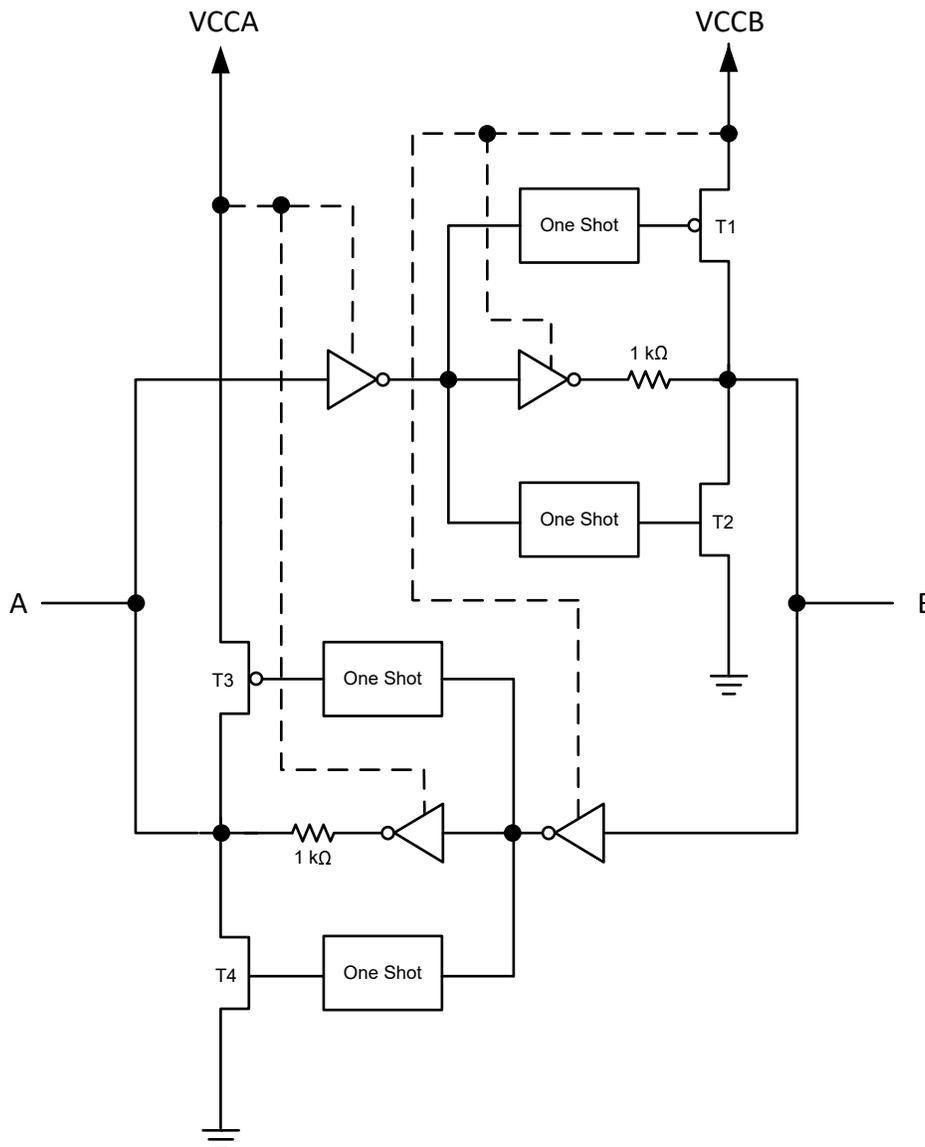
**Figure 7-1. Architecture of TXB0604 Device I/O Cell**
