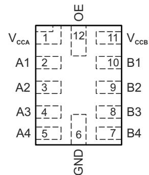
**Figure 4-4. RUT Package, 12-Pin UQFN (Top View)**
