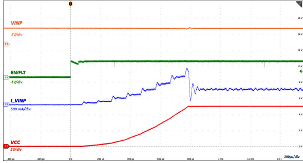
Figure 6-25. Start-Up with En/FLT From Low to High: VINP = 5.0V , VCC = 5.0V , 18Ω Load
