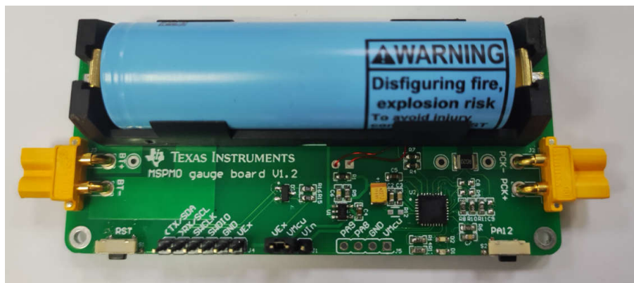
Figure 5-2. MSPM0 Gauge Hardware Board
