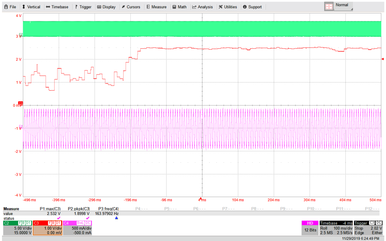
Figure 4-19. Steady Count Change When Q1 Regulation is Lost
