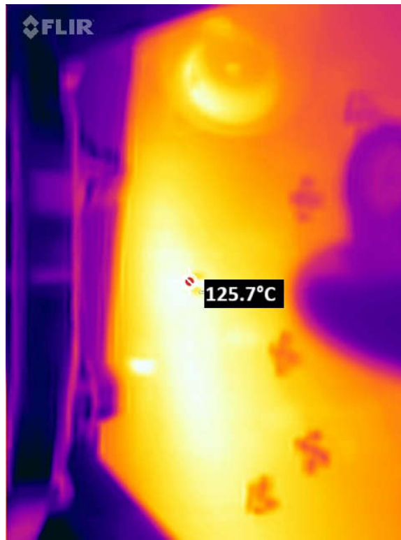
Figure 4-3. SN54SC1G125-SEP Thermal Image for SEL
