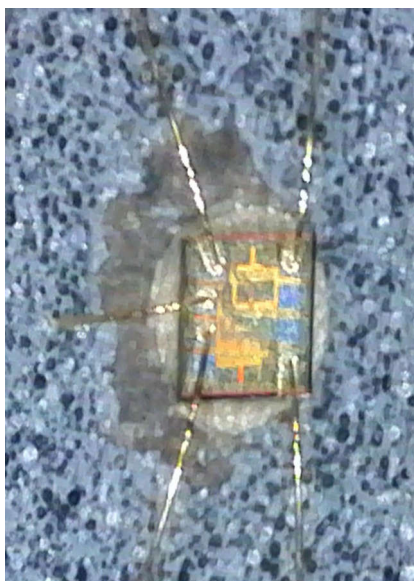
Figure 3-2. Photo of SN54SC1G125-SEP Package Decapped
