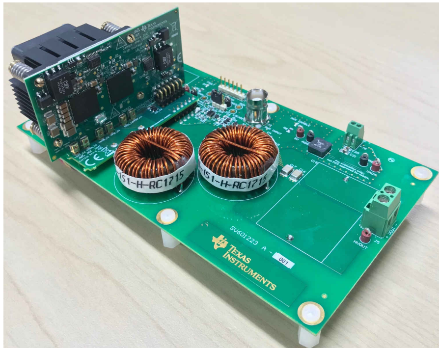
Figure 8-1. LMG342XEVM-04X Connected to the LMG34XX-BB-EVM
