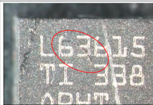
Figure 3. Unit 1. Blown package in area of pin 12
