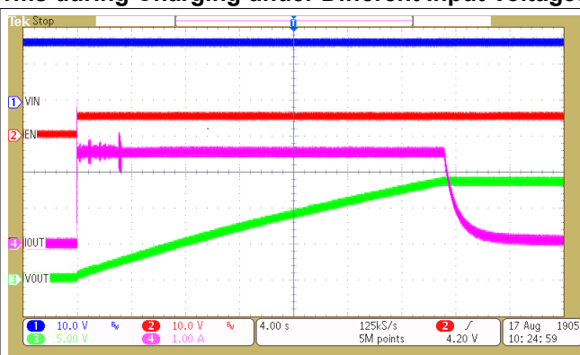
Figure 4-3. Charging Process at VIN = 16V
