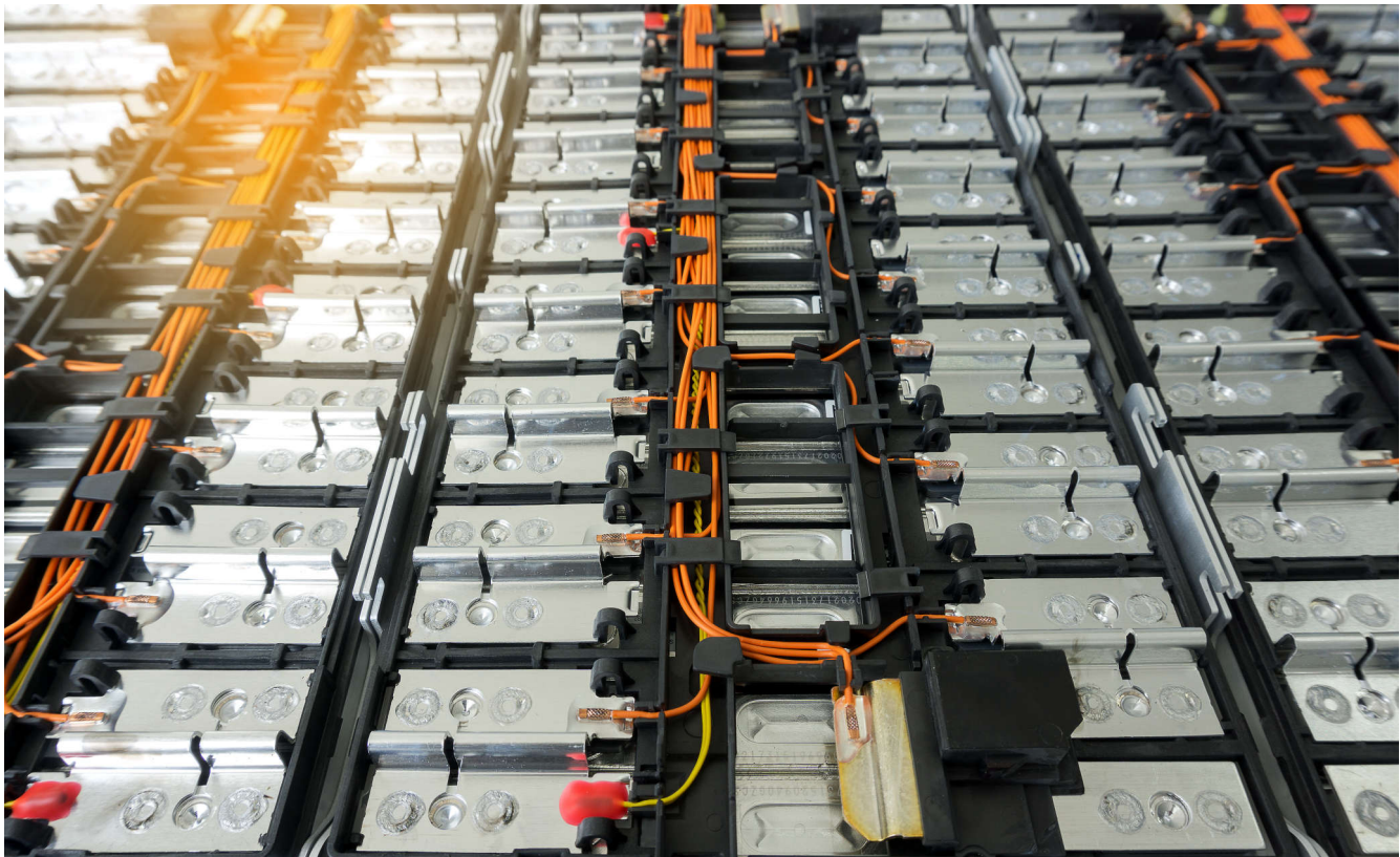
Figure 3-1. Lithium Cells in an EV Battery Pack
