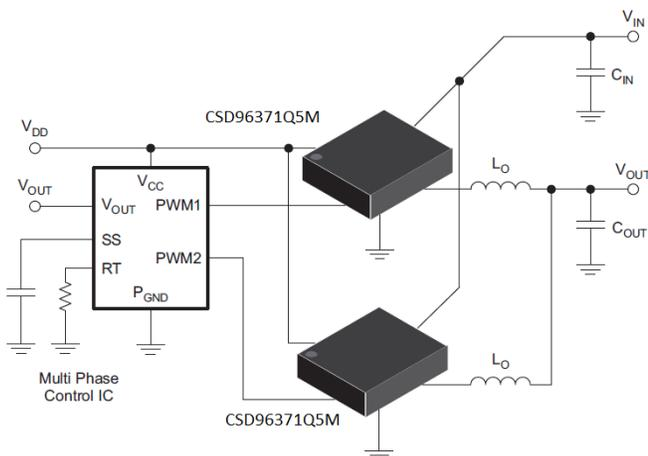
Figure 1. Application Diagram
