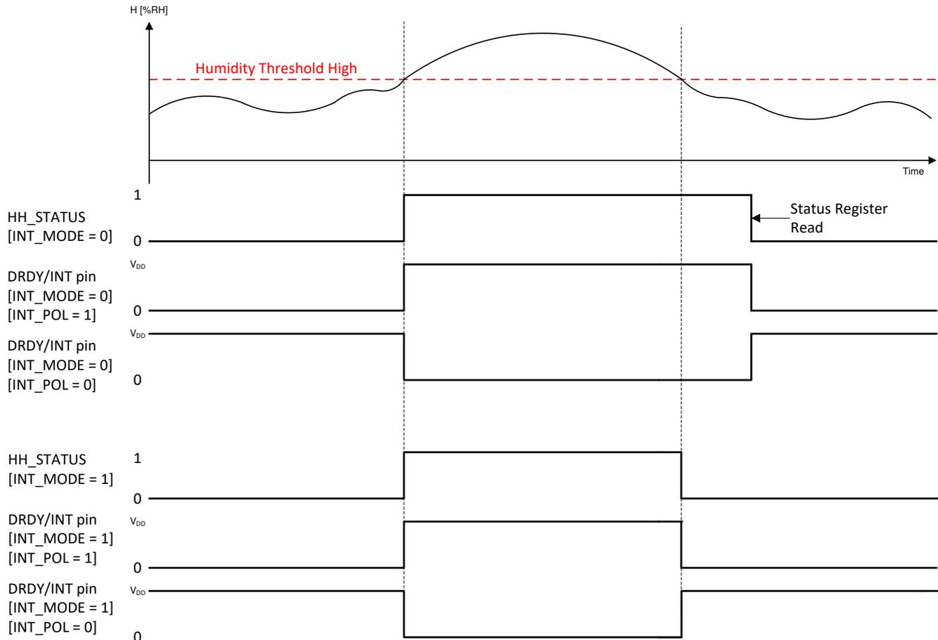
Figure 7-5. INTERRUPT on Threshold - Humidity High
