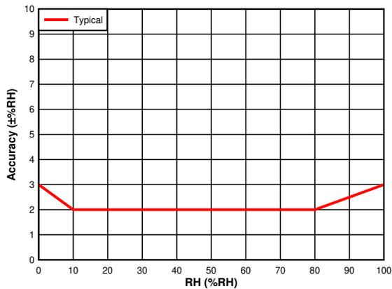
Figure 6-2. RH Accuracy vs. RH Set Point
