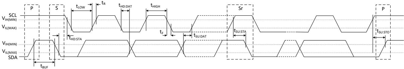
**Figure 6-1. I<sup>2</sup>C Timing Diagram**
