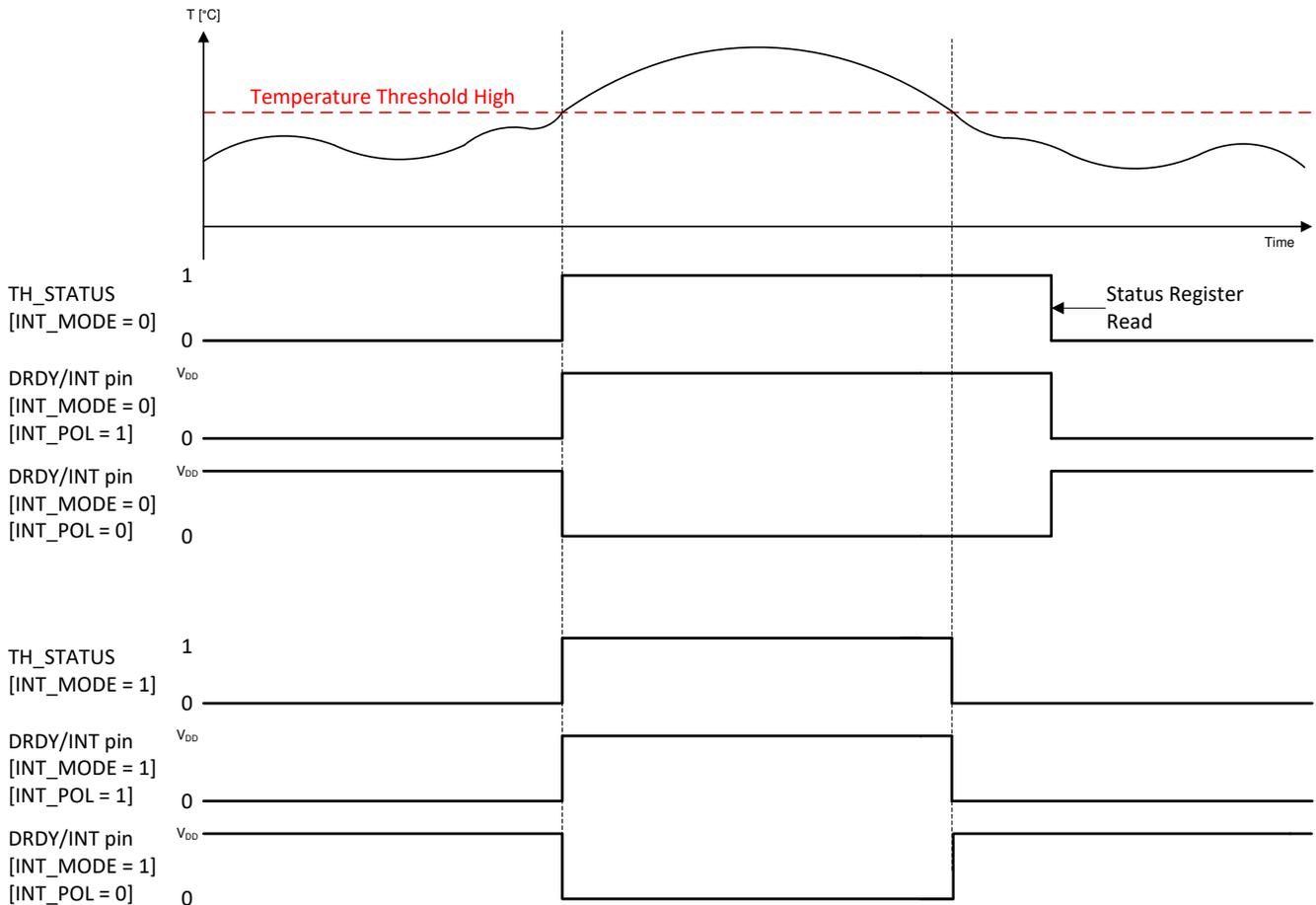
Figure 7-3. INTERRUPT on Threshold - Temperature High
