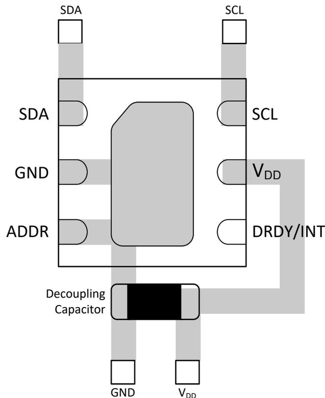
TI does NOT recommend to solder the thermal pad to PCB to achieve faster heating response if the integrated heater is used.
