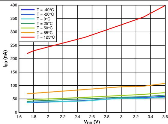
Figure 6-6. Supply Current vs. Supply Voltage, Sleep Mode
