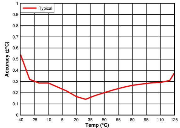
Figure 6-3. Temperature Accuracy vs. Temperature Set Point
