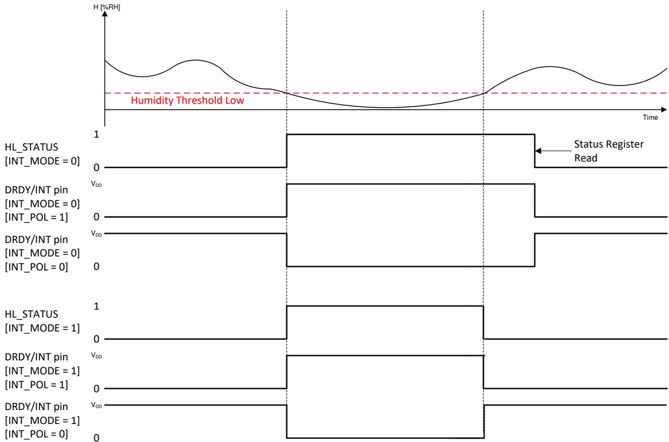
**Figure 7-6. INTERRUPT on Threshold - Humidity Low**
