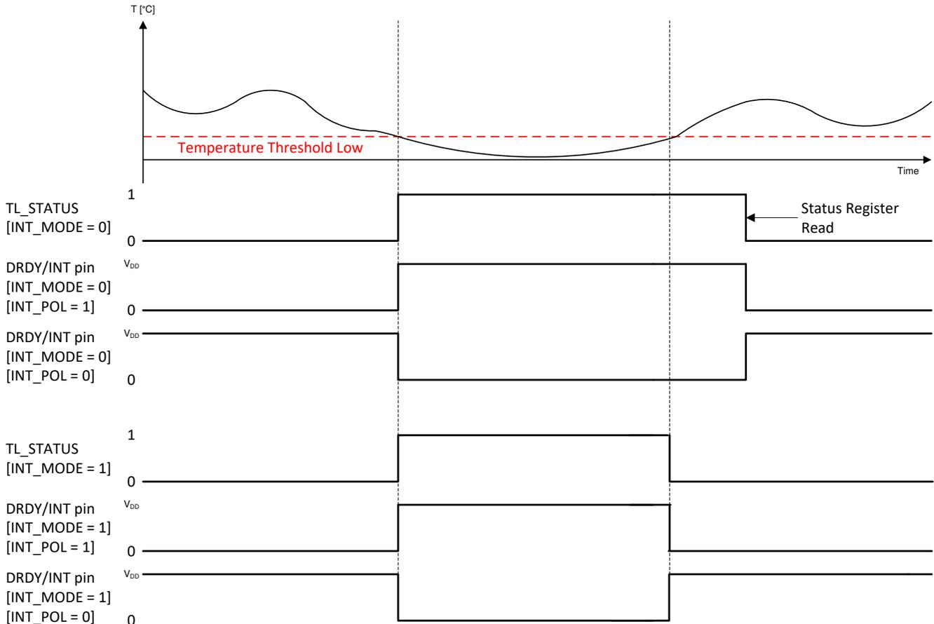
**Figure 7-4. INTERRUPT on Threshold - Temperature Low**
