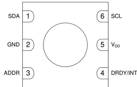
**Figure 5-1. DEP Package 6-Pin WSON Transparent Top View**
