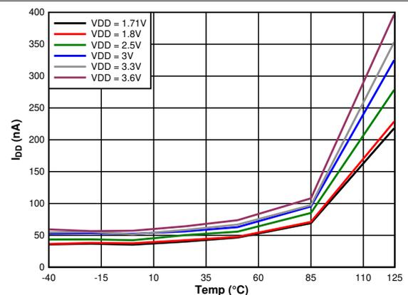
Figure 6-7. Supply Current vs. Temperature, Sleep Mode
