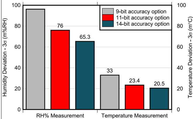
Figure 6-10. Average Measurement Sensitivity vs. Accuracy Option
