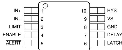
**Figure 5-2. DGS Package 10-Pin VSSOP Top View**
