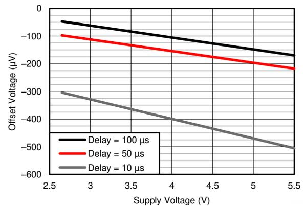
**Figure 6-4. Input Offset Voltage vs Supply Voltage**
