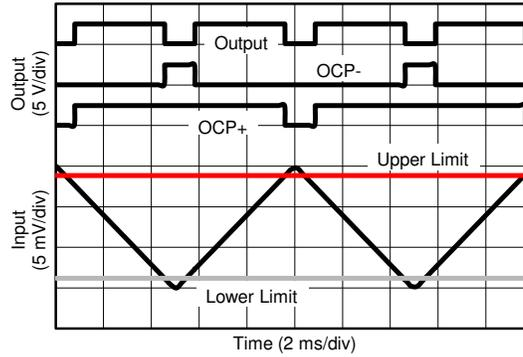
**Figure 8-6. Output Waveform**
