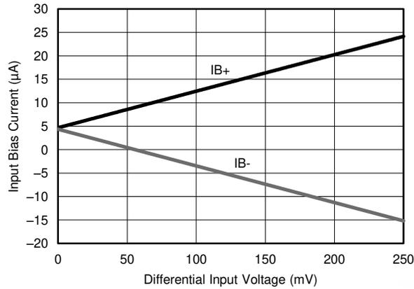
Figure 7-10. Input Bias Current vs Differential Input Voltage
