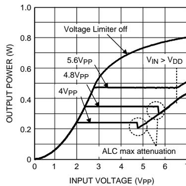
**Figure 25. Voltage Limiter Function**
