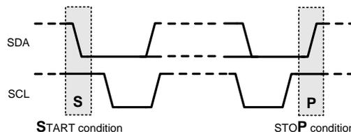
Figure 21. Example I<sup>2</sup>C Write Cycle
