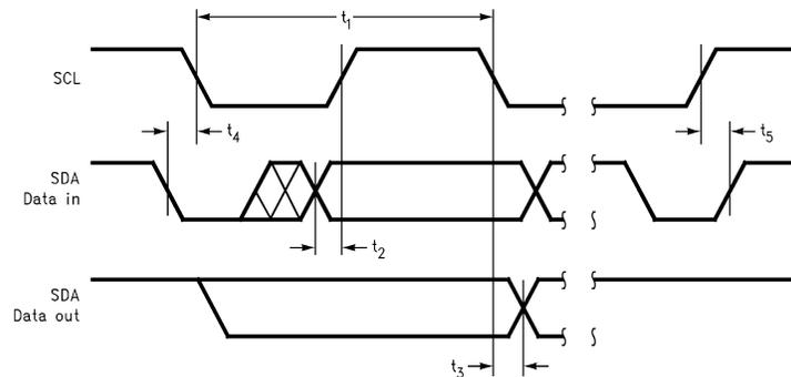
Figure 20. I<sup>2</sup>C Timing Diagram
