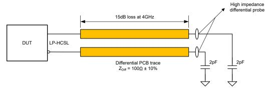
Figure 6-2. LP-HCSL PCle AC Test Load
