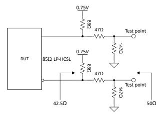
Figure 6-3. LP-HCSL DC Simulation Load
