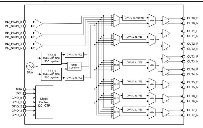
Figure 7-2. LMK3H2108 Functional Block Diagram
