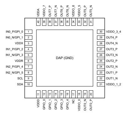
Figure 4-2. LMK3H2108 RKP Package 40-Pin QFN Top View
