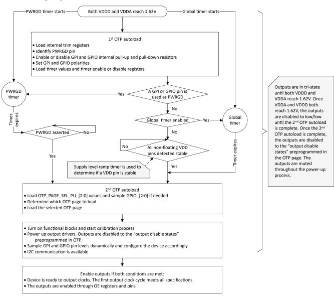
Figure 7-3. LMK3H2108 Power Up Sequence
