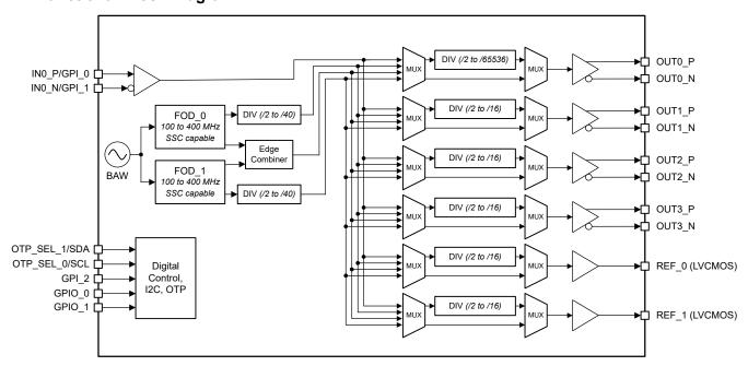
Figure 7-1. LMK3H2104 Functional Block Diagram
