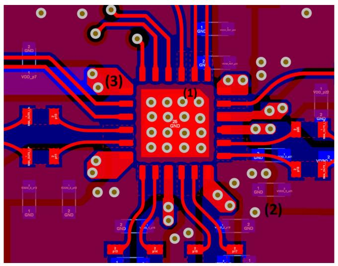
Figure 8-6. LMK3H2104 Top and Bottom Layers Example Layout
