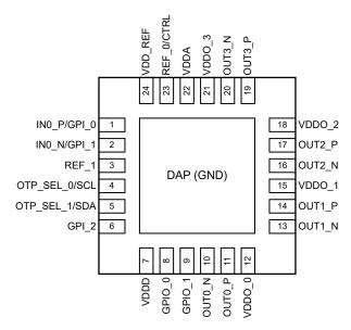
Figure 4-1. LMK3H2104 RGE Package 24-Pin QFN Top View
