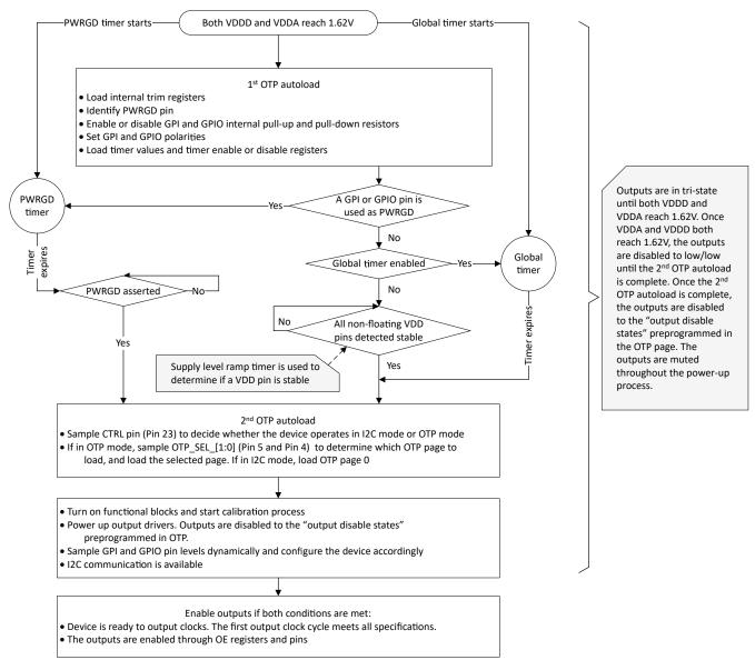
Figure 7-4. LMK3H2104 Power Up Sequence
