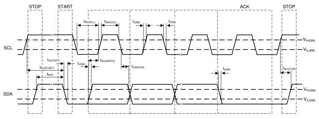
Figure 7-10. I<sup>2</sup>C Timing Diagram
