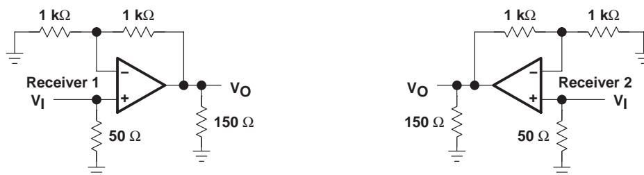
Figure 2. Receiver Input-to-Output Crosstalk Test Circuit
