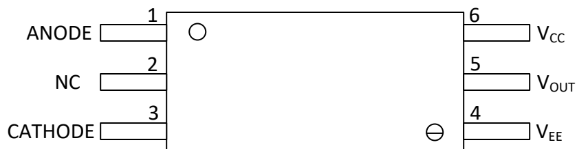
Figure 5-1. UCC23313 Package SO-6 Top View
