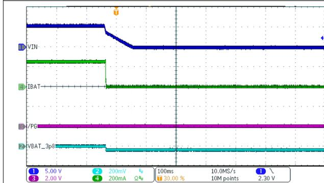
$V_{IN} = 5 \text{ V} \rightarrow 0 \text{ V}$
