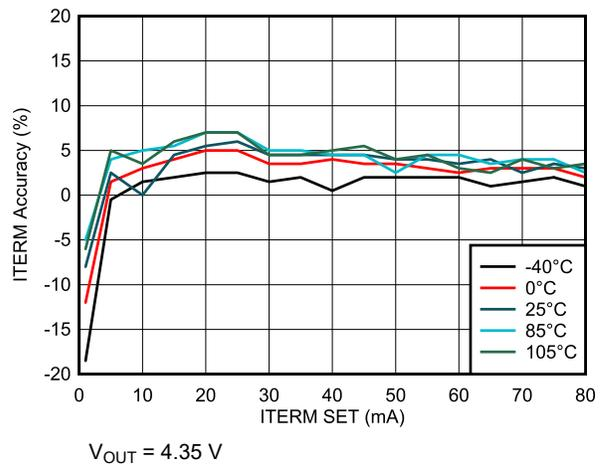
**Figure 6-10. Termination Current Accuracy vs. Termination Current Setting**
