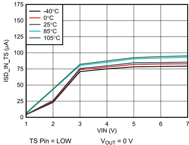
**Figure 6-7. Input Shutdown Current vs. Input Voltage**
