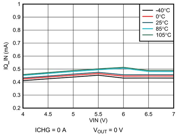
**Figure 6-8. Input Quiescent Current vs. Input Voltage**
