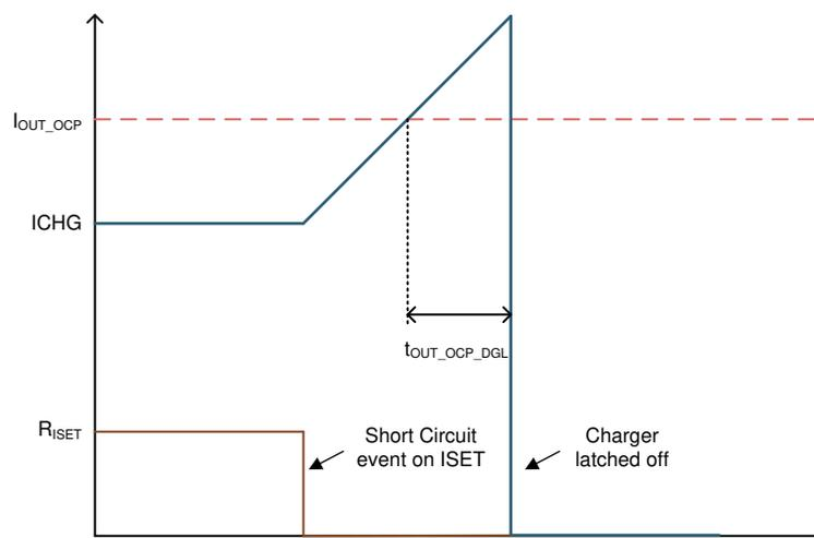
**Figure 7-4. Overcurrent Protection**
