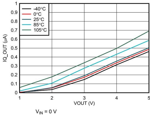
**Figure 6-9. Output Quiescent Current vs. Output Voltage**
