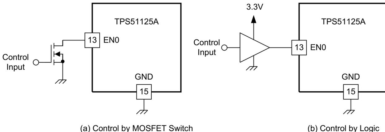
Figure 38. Control Example of EN0 Master Enable
