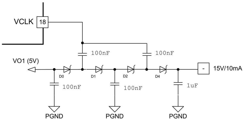
Figure 39. 15-V / 10-mA Charge Pump Configuration
