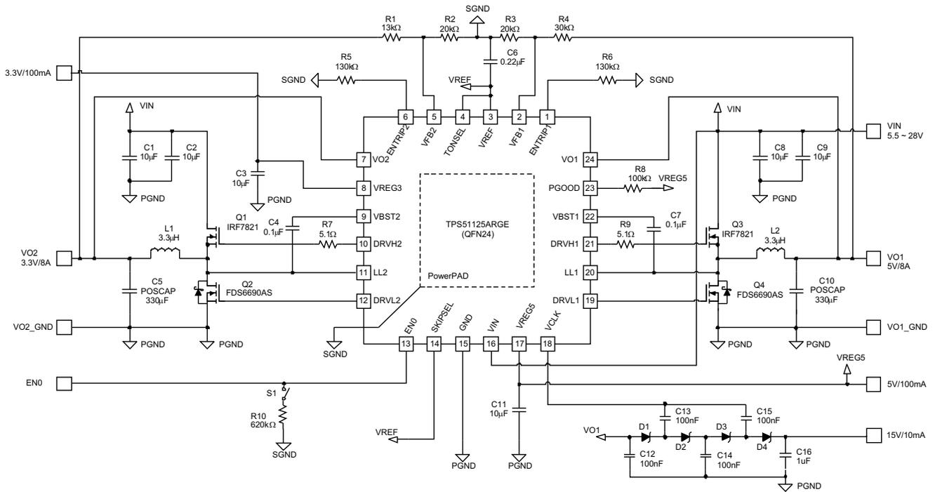
Figure 42. 5-V/8-A, 3.3-V/8-A Application Circuit (245-kHz/305-kHz Setting)
