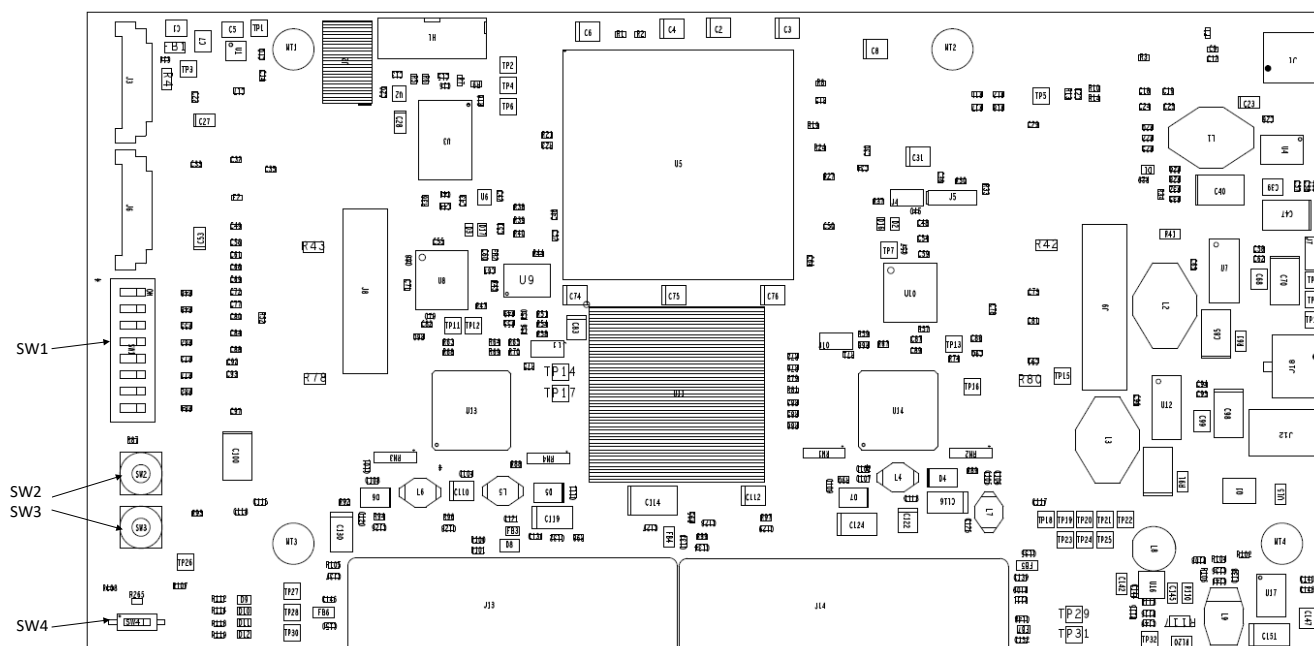
Figure 2-5. DLPLCRC410EVM On-Board Switches
