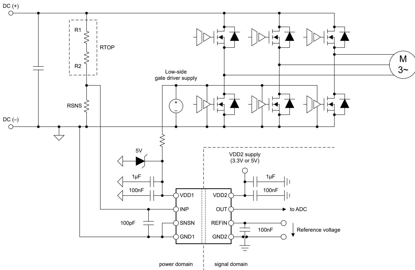
Figure 8-1. Using the AMC0x11R-Q1 in a Typical Application
