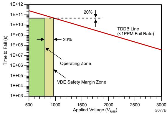
$T_A$  up to 150°C, stress-voltage frequency = 60Hz, isolation working voltage = 800V<sub>RMS</sub>, projected operating lifetime  $>> 100$  years
