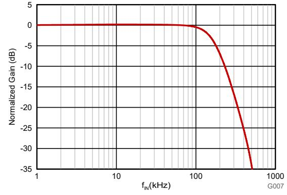
Figure 6-11. Normalized Gain vs Input Frequency
