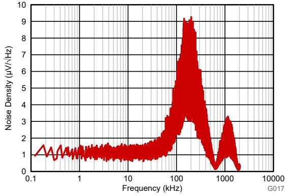
Figure 6-10. Input-Referred Noise Density vs Frequency
