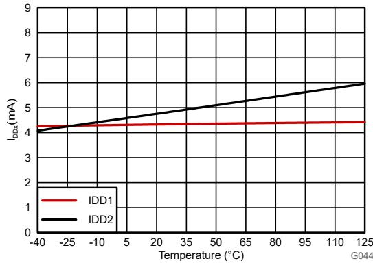
Figure 6-14. Supply Current vs Temperature
