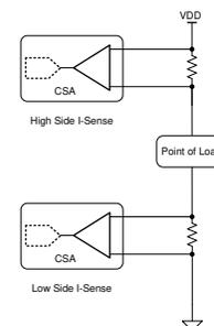
Figure 2. Point of Load Current Sensing Options
