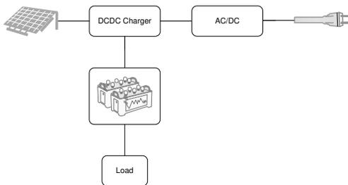
Figure 1. WI Power Supply Block Diagram
