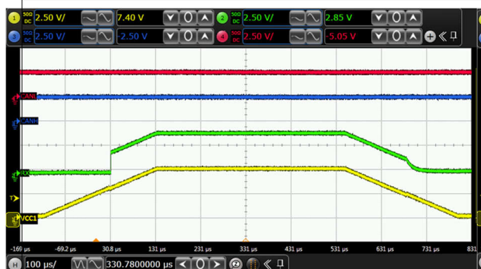
Figure 5-13. Glitch Free Power Up on V_{CC1} – CAN Bus Remains Recessive
