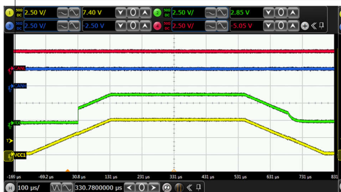
Figure 5-13. Glitch Free Power Up on V_{CC1} – CAN Bus Remains Recessive
