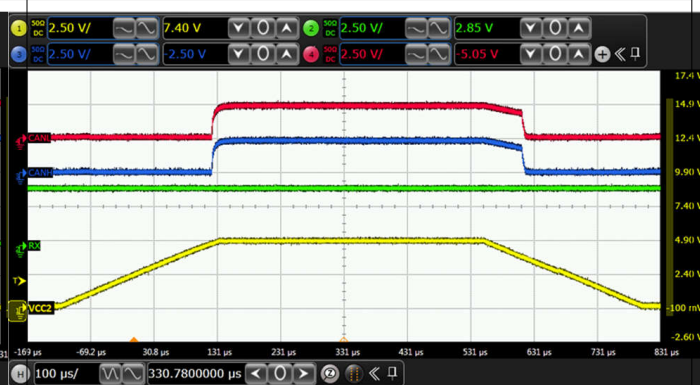
Figure 5-12. Typical TXD, RXD, CANH and CANL Waveforms at 1Mbps
