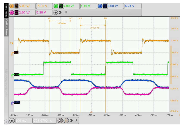
Figure 6-16. Typical TXD, RXD, CANH and CANL Waveforms at 5Mbps
