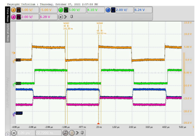
Figure 6-14. Typical TXD, RXD and CANL Waveforms at 500kbps
