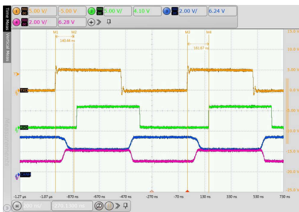
Figure 6-15. Typical TXD, RXD, CANH and CANL Waveforms at 2Mbps
