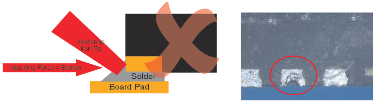
Figure 6-4. Manual Rework Damage
