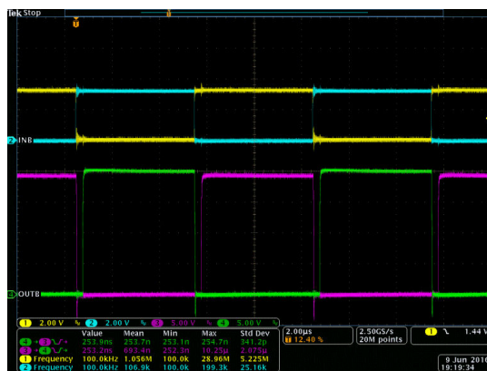
Figure 8-5. Bench Test Waveform for INA/B and OUTA/B
