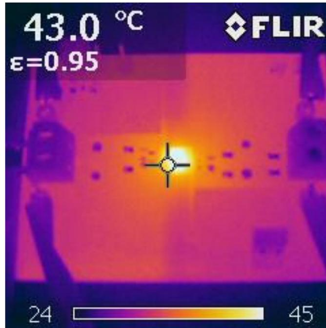
Figure 3-14.  $V_{INP}=5\text{ V}$ ,  $I_{LOAD}=150\text{mA}$ ,  $P_{out}=0.75\text{W}$
