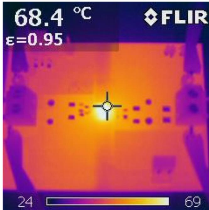
Figure 3-13. VINP=5.0V, I<sub>VCC</sub>=300mA, P<sub>out</sub>=1.5W
