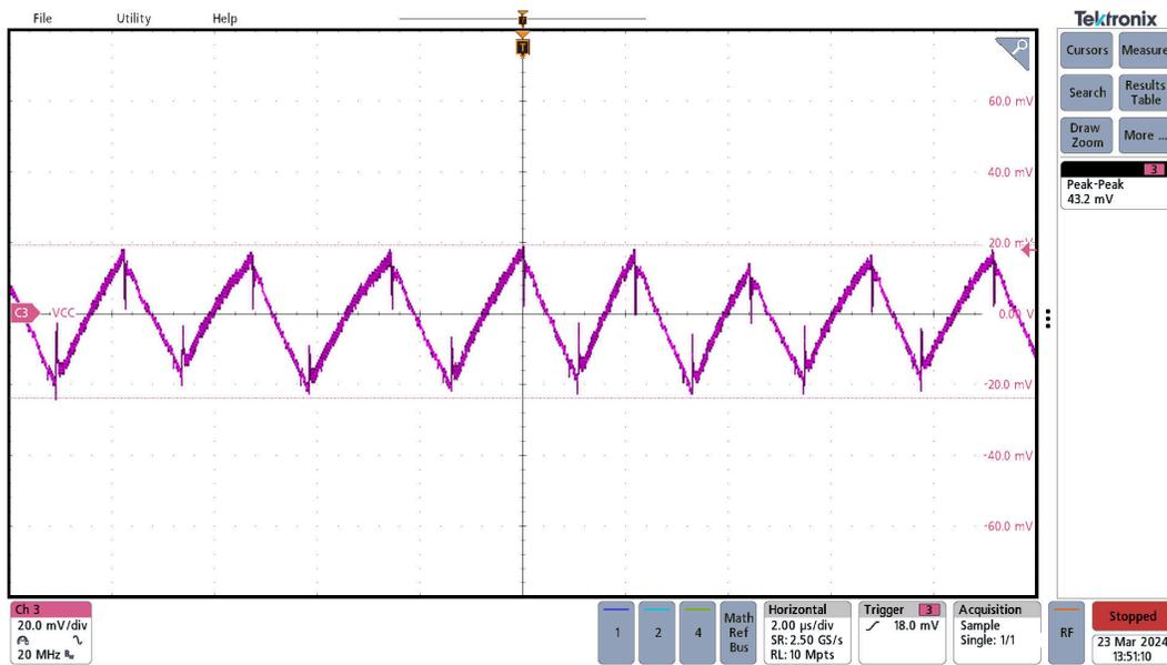
Figure 3-9. VISO AC Ripple:  $V_{pkpk} = 56$  mV,  $V_{INP} = 5$  V,  $V_{ISO} = 5$  V,  $I_{LOAD} = 300$  mA
