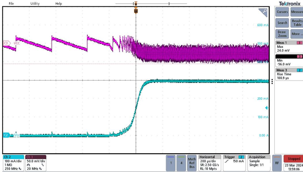
Figure 3-10. Load transient, VINP=5.0V, VCC=5.0V, No load ( $I_{LOAD}=0\text{mA}$ ) to Full load ( $I_{LOAD}=300\text{mA}$ )
