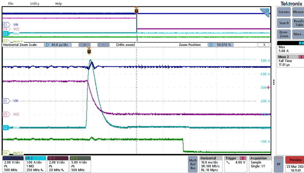
Figure 3-12. Short circuit, VINP=5.0V, VCC=5.0V
