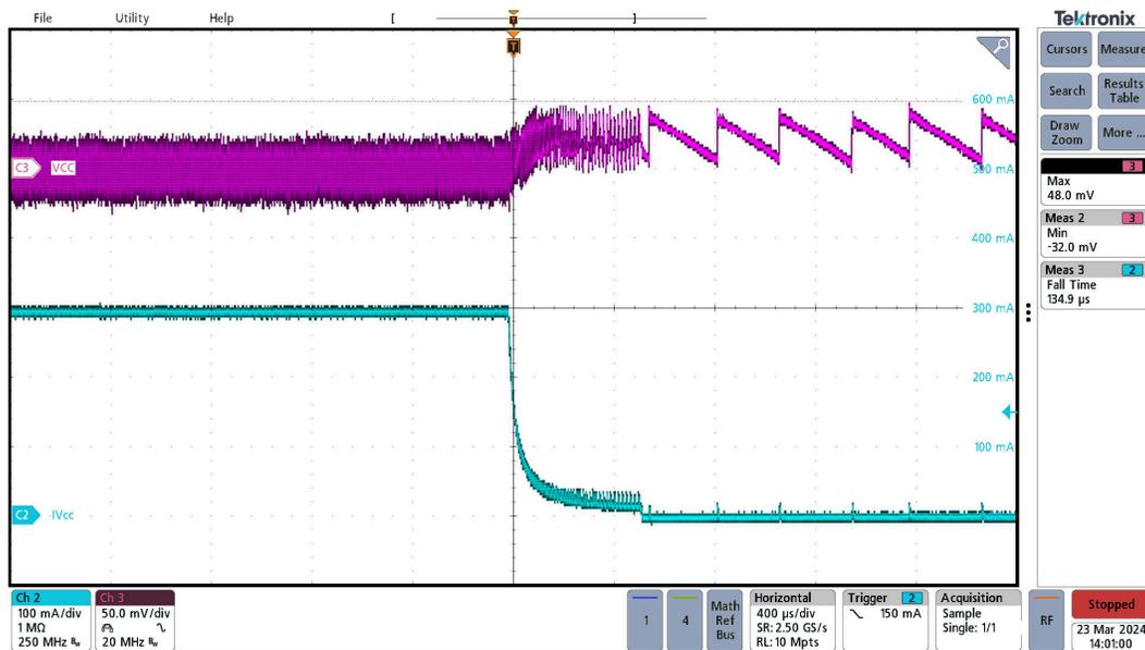
Figure 3-11. Load transient, VINP=5.0V, VCC=5.0V, Full load ( $I_{LOAD}=300\text{mA}$ ) to No load ( $I_{LOAD}=0\text{mA}$ )
