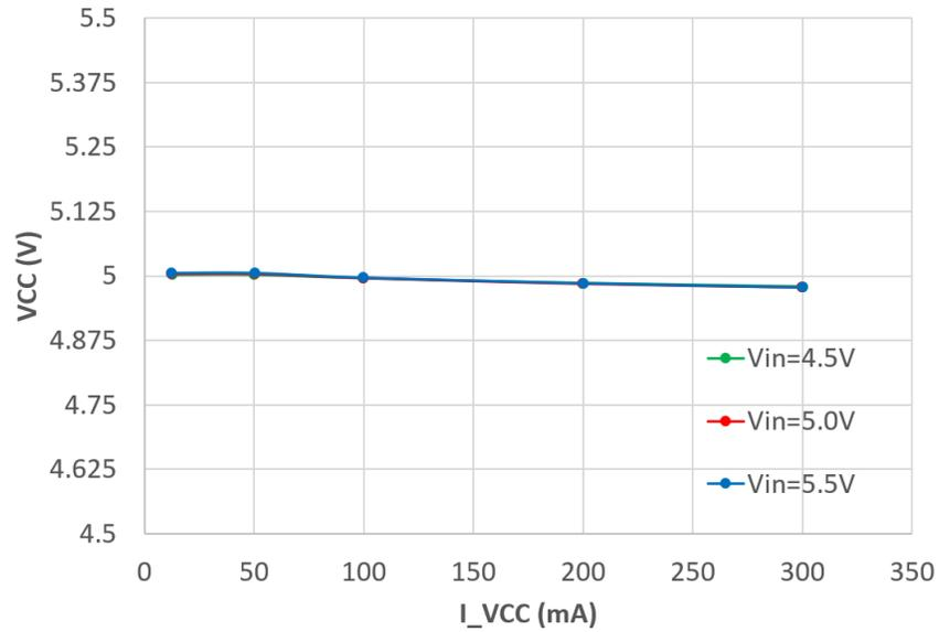
**Figure 3-3. Regulation vs Load Current**
