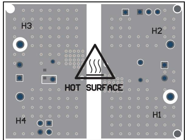
**Figure 4-6. PCB Bottom Layer, Assembly (Mirrored View)**
