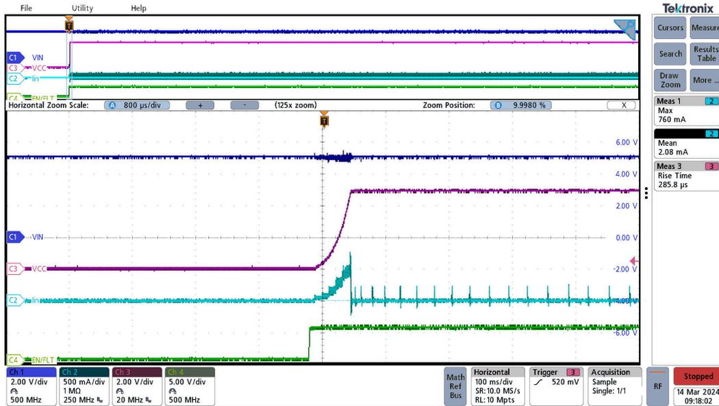
Figure 3-6. Inrush current VINP=5.0V, VCC=5.0V, I<sub>LOAD</sub>=0mA, Toggling EN
