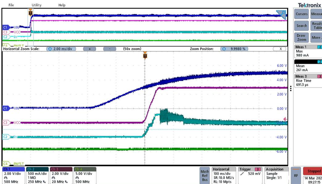
Figure 3-5. Start-up  $V_{INP}=5.0V$ ,  $V_{CC}=5.0V$ , Full load ( $R_{load}=18\Omega$ ),  $EN=5.0V$
