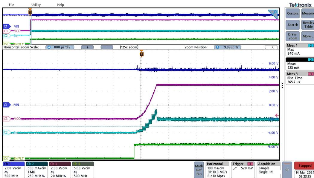
Figure 3-7. Inrush current VINP=5.0V, VCC=5.0V, Full load (R<sub>load</sub>=18Ω), Toggling EN
