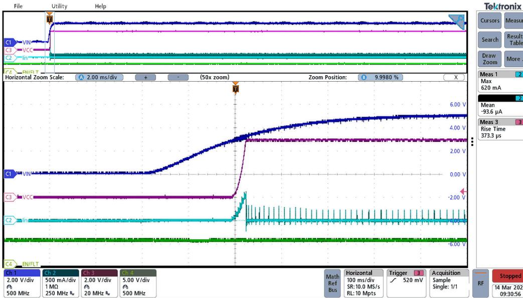
Figure 3-4. Start-up  $V_{INP}=5.0V$ ,  $V_{CC}=5.0V$ ,  $I_{LOAD}=0mA$ ,  $EN=5.0V$
