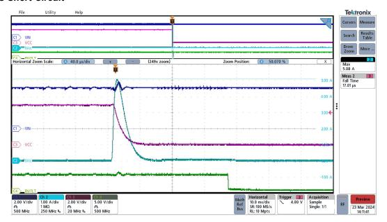
Figure 3-12. Short circuit, VINP=5.0V, VCC=5.0V
