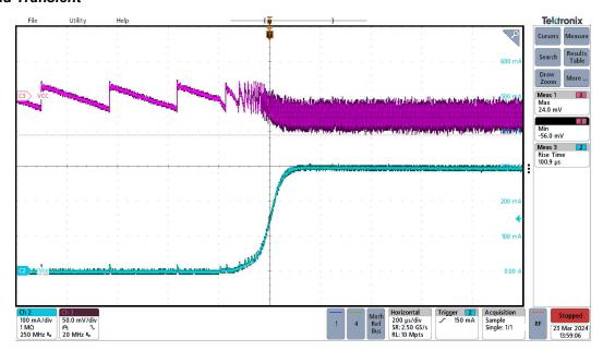
Figure 3-10. Load transient, VINP=5.0V, VCC=5.0V, No load (I<sub>LOAD</sub>=0mA) to Full load (I<sub>LOAD</sub>=300mA)
