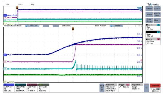
Figure 3-4. Start-up VINP=5.0V, VCC=5.0V, I<sub>LOAD</sub>=0mA, EN=5.0V
