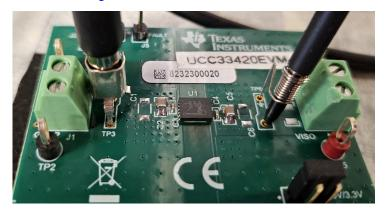
Figure 2-2. PCB Scope Probe Test Points
