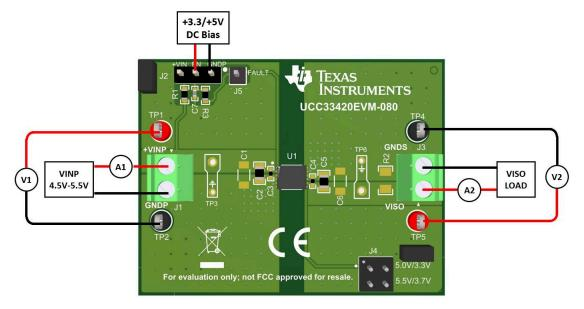
Figure 2-1. Typical Efficiency Measurement Setup
