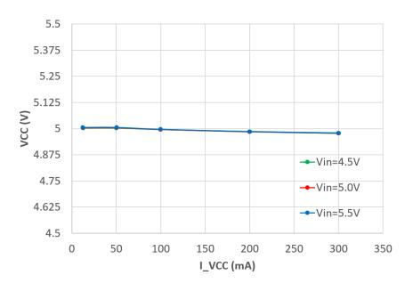
Figure 3-3. Regulation vs Load Current
