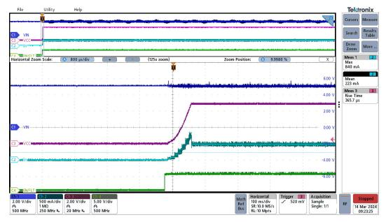
Figure 3-7. Inrush current VINP=5.0V, VCC=5.0V, Full load (Rload=18Ω), Toggling EN
