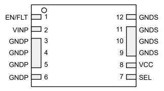
Figure 1-1. UCC33420-Q1 Package (Top View)
