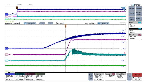
Figure 3-5. Start-up VINP=5.0V, VCC=5.0V, Full load (Rload=18Ω), EN=5.0V
