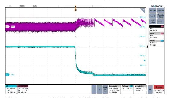
Figure 3-11. Load transient, VINP=5.0V, VCC=5.0V, Full load ( $I_{LOAD}$ =300mA) to No load ( $I_{LOAD}$ =0mA)
