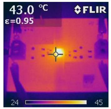
Figure 3-14. VINP=5 V,  $I_{LOAD}$ =150mA, Pout=0.75W
