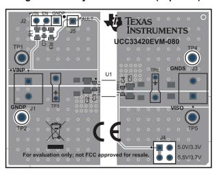
Figure 4-3. PCB Top Layer, Assembly
