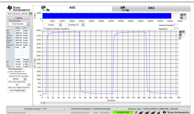
Figure 8-7. 40MHz, Square-Wave Time Domain for 5GSPS, Single-Channel Oscilloscope
