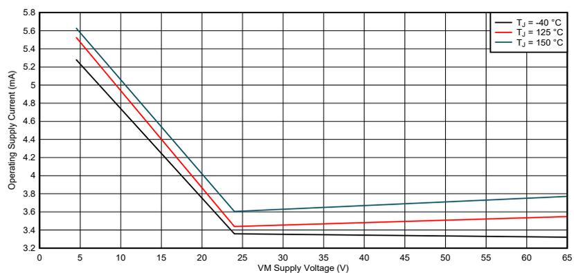
Figure 6-3. Operating supply current, VCC = External 5 V
