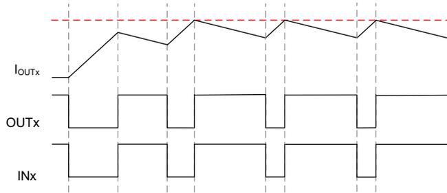
**Figure 7-7. Inductive Load Connected to VM, Cycle-by-cycle control**
