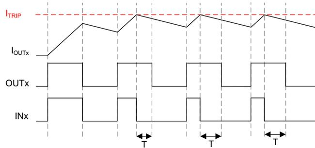
**Figure 7-6. Inductive Load Connected to ground, Cycle-by-cycle control**
