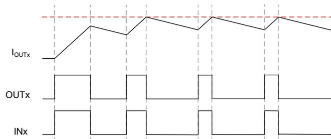
**Figure 7-5. Inductive Load Connected to ground, Cycle-by-cycle control**
