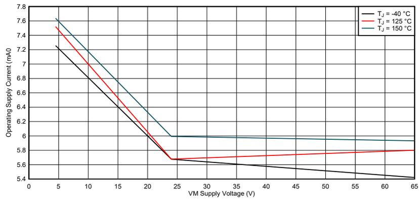
Figure 6-4. Operating supply current, VCC = DVDD
