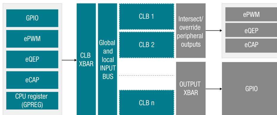
**Figure 4-4. CLB Integration in C2000 MCU Architecture**
