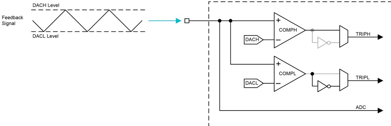
**Figure 2-3. CMPSS Block Diagram**
