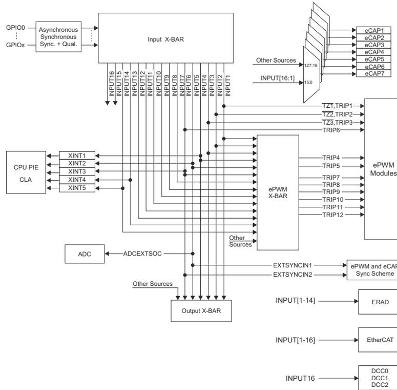
**Figure 3-7. Input X-Bar on the TMS320F2837xD MCU**
