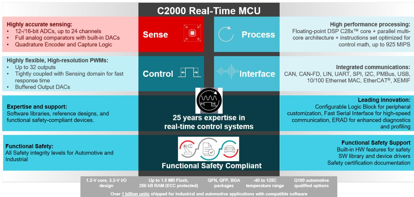
Figure 1-2. C2000 Real-Time MCU Components
