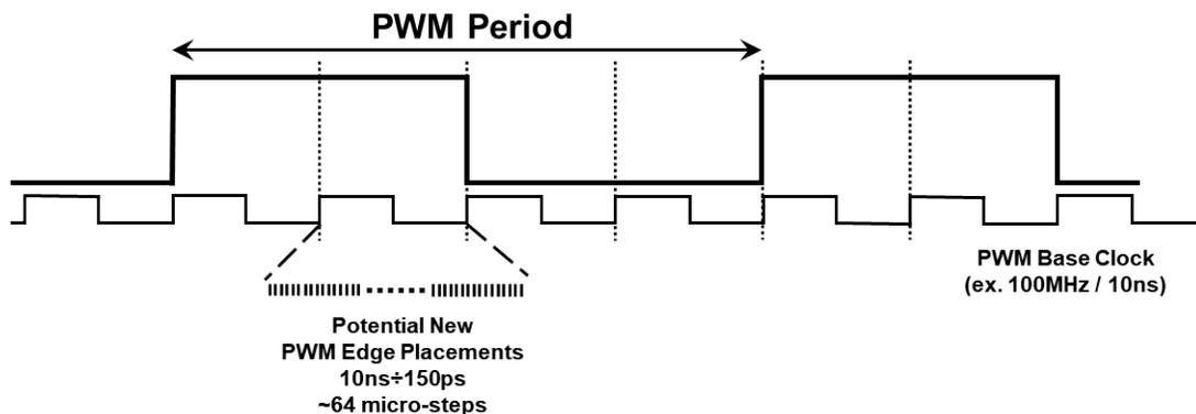
**Figure 4-1. HRPWM Capability vs Traditional PWM Generation Methods**
