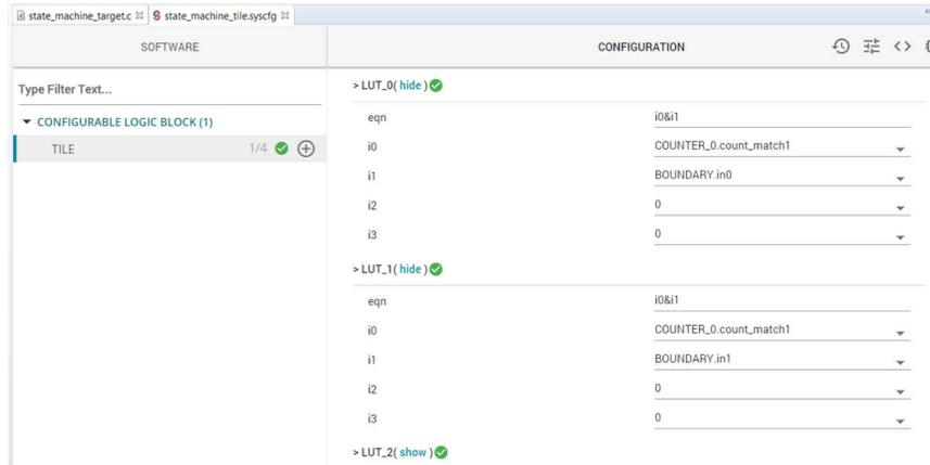
**Figure 4-5. CLB Configuration Tool in SysConfig**
