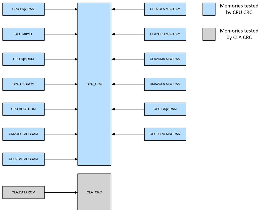
**Figure 6-3. BGCRC Implementation on the TMS320F2838xD Device**
