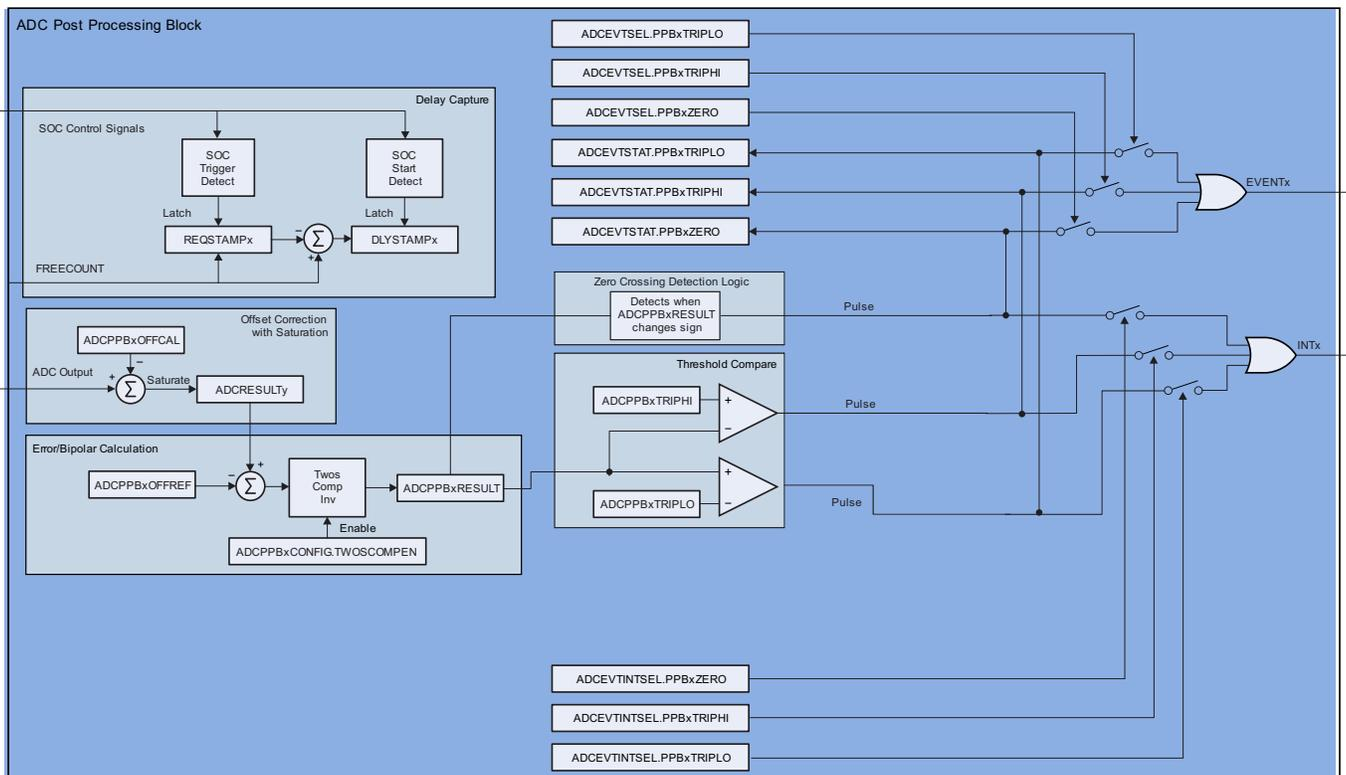
**Figure 2-4. ADC Post Processing Block on TMS320F2837xD**
