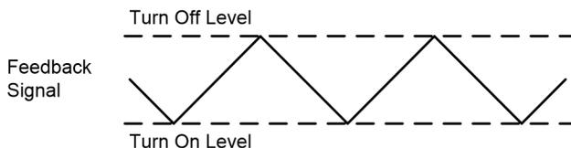
**Figure 2-2. Threshold Levels in a Hysteresis Controller**
