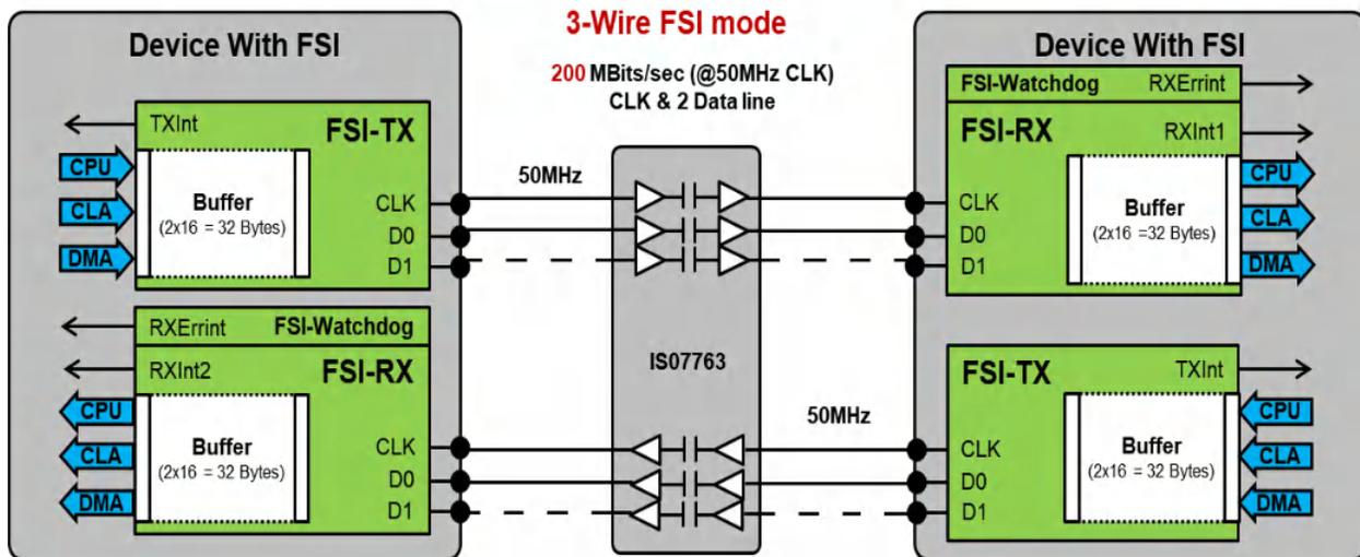
The TX and RX ports work asynchronously to each other.
