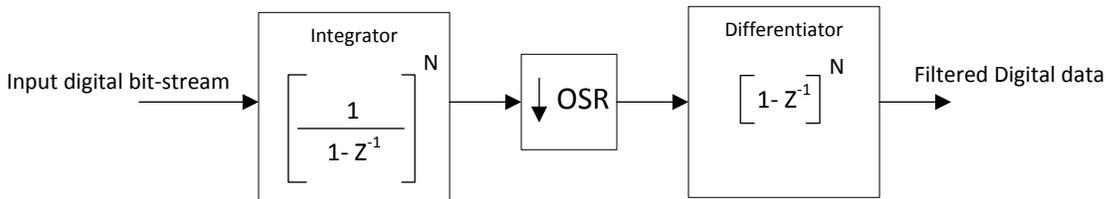
Figure 2-7. Filter and Demodulator Inside the C2000 SDFM
