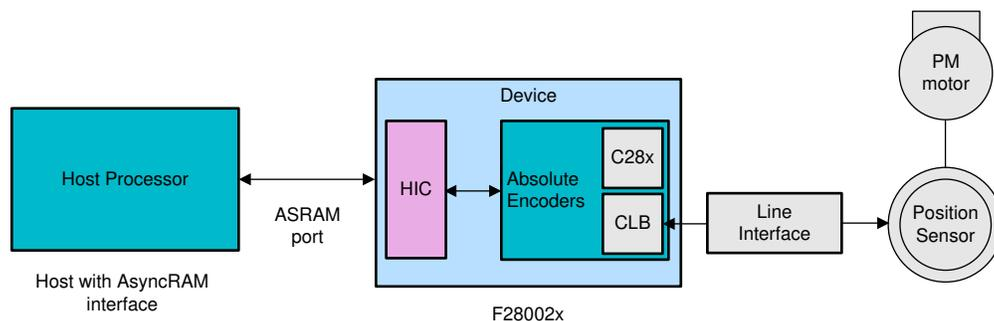
**Figure 5-2. HIC Bridge for Position Encoder Applications**
