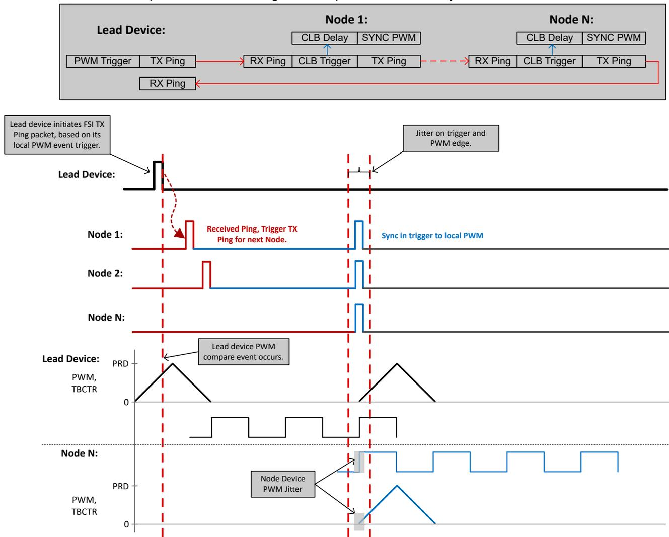
Figure 4-11. Daisy Chain Network Synchronization and Timing
