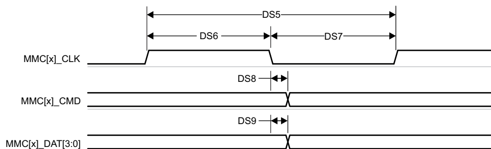
Figure 6-101. MMC1/2 – Default Speed – Transmit Mode
