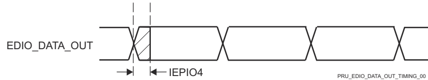
Figure 6-101. PRU_ICSSG IEP Digital IOs Timing Requirements
