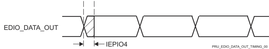
Figure 6-101. PRU_ICSSG IEP Digital IOs Timing Requirements
