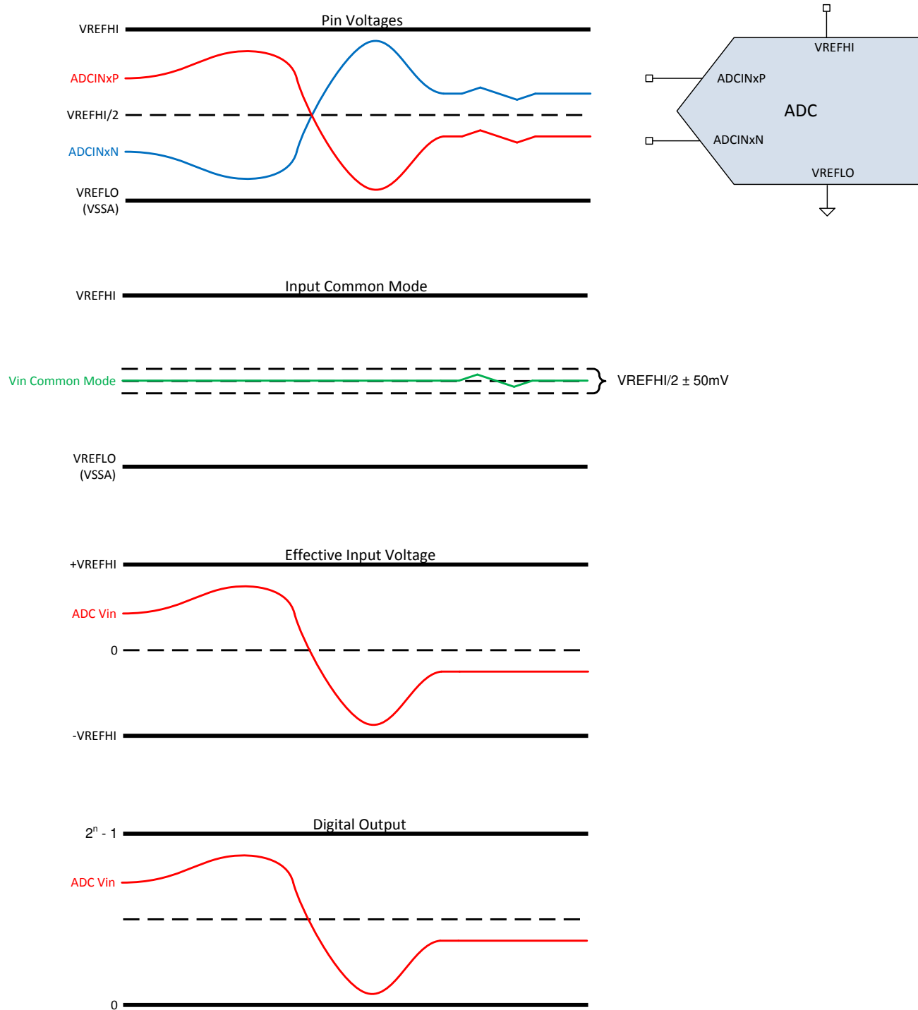
Figure 6-36. Differential Signaling Mode
