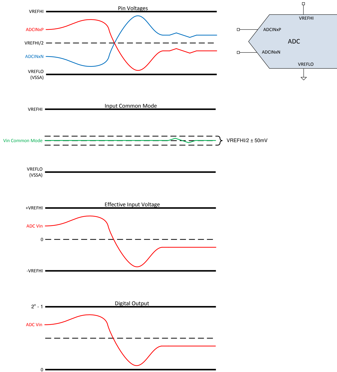
Figure 6-36. Differential Signaling Mode
