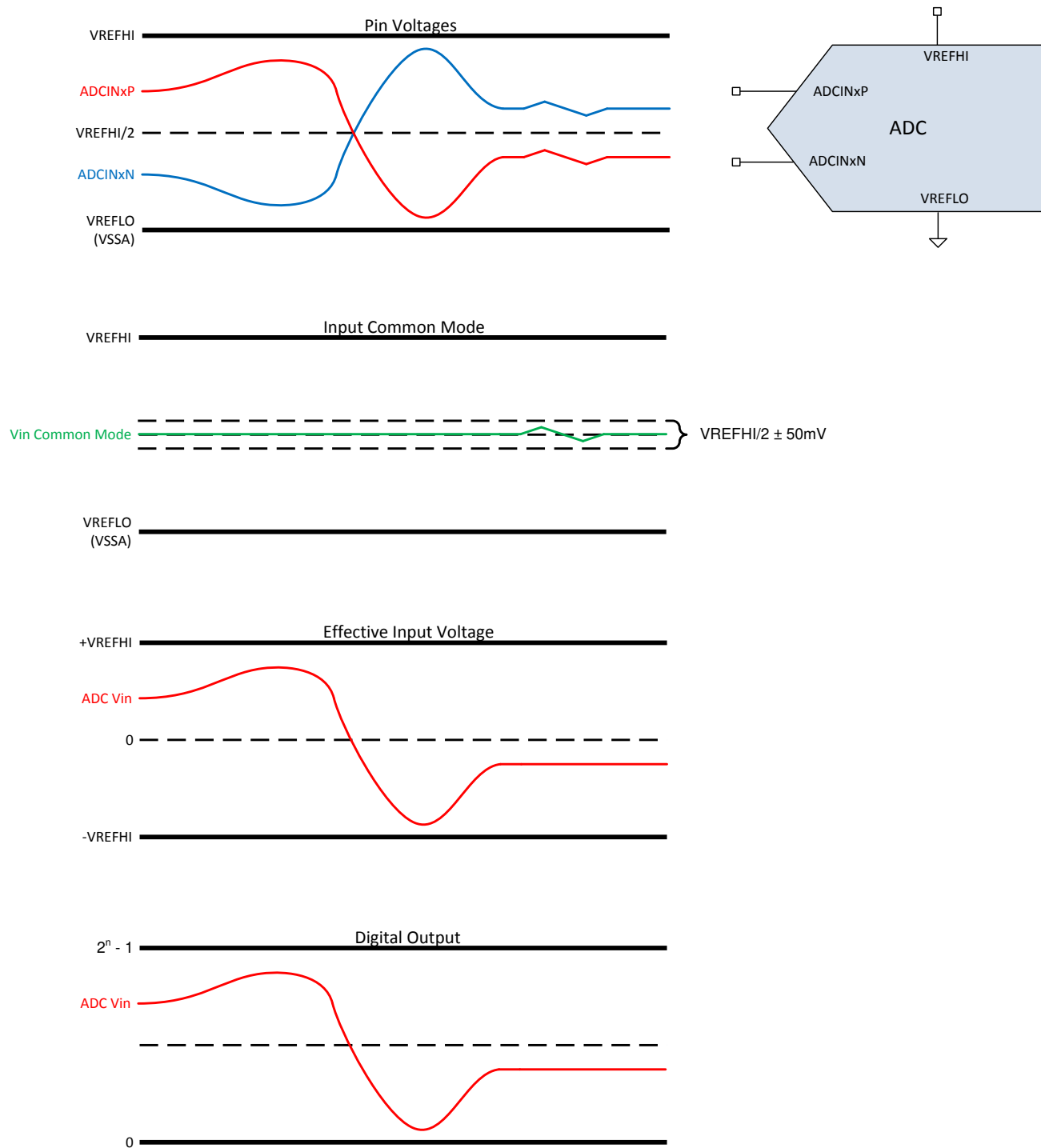
Figure 6-36. Differential Signaling Mode
