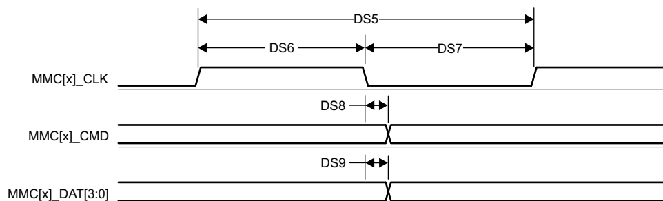
Figure 6-90. MMC1 – Default Speed – Transmit Mode
