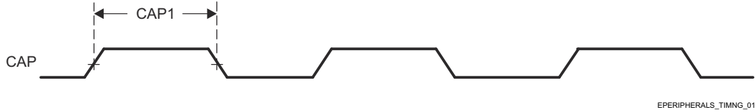
Figure 6-46. eCAP Input Timings
