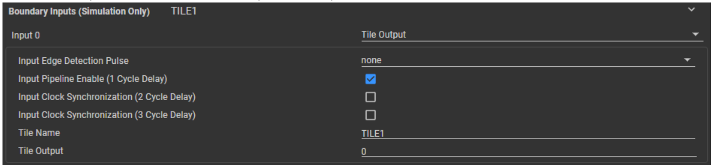
Figure 3-19. Boundary Input Tile Output
