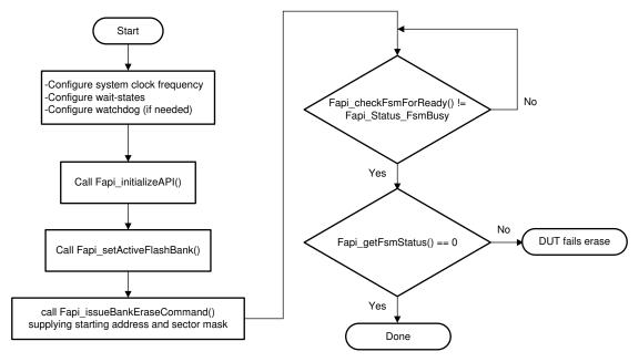
Figure 4-2. Recommended Bank Erase Flow
