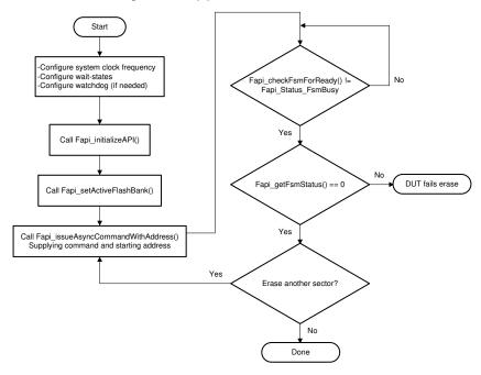
Figure 4-1. Recommended Erase Flow
