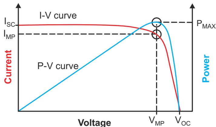
**Figure 2-7. Solar Panel Characteristics I-V and P-V Curves**
