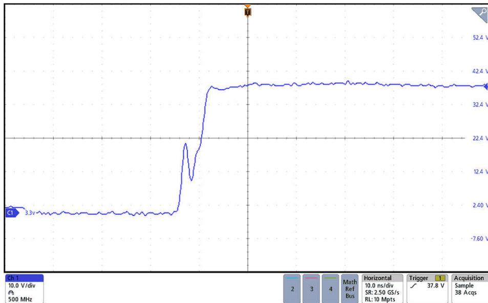
Figure 3-7. Switch Nodes at 40V Input; 24V, 16A Output, rising edge
