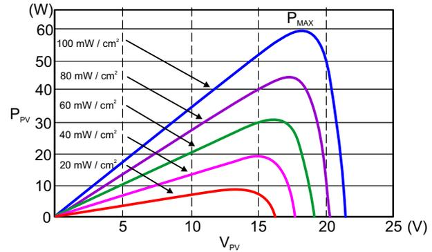
**Figure 2-9. Solar Panel Output Power Variation Under Different Irradiation Conditions—Graph B**
