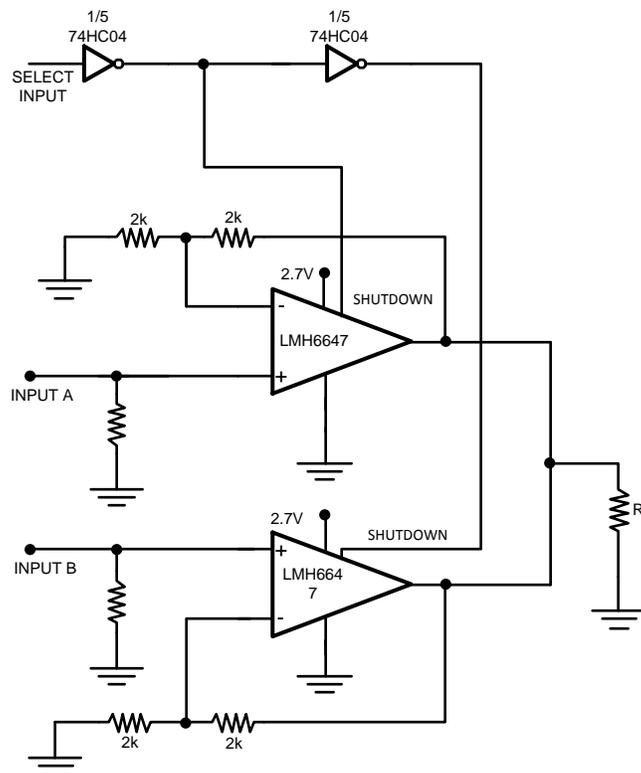
**Figure 46. 2:1 MUX Operating off a 2.7V Single Supply**
