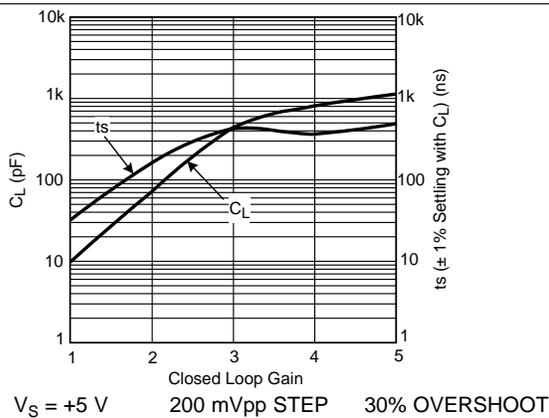
Figure 17. Cap Load Tolerance and Setting Time vs. Closed Loop Gain
