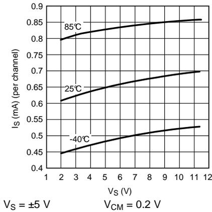
Figure 33.  $I_S$  (mA) vs.  $V_S$ (V)
