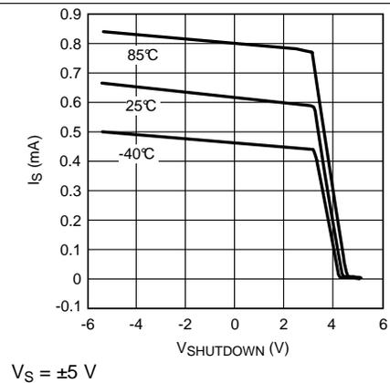
Figure 36.  $I_S$  vs.  $V_{SHUTDOWN}$  (LMH6647)
