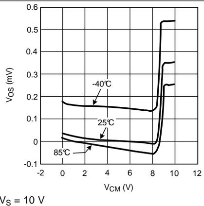
Figure 28.  $V_{OS}$  vs.  $V_{CM}$  (a Typical Unit)
