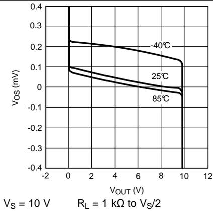
Figure 25.  $V_{OS}$  vs.  $V_{OUT}$  (a Typical Unit)
