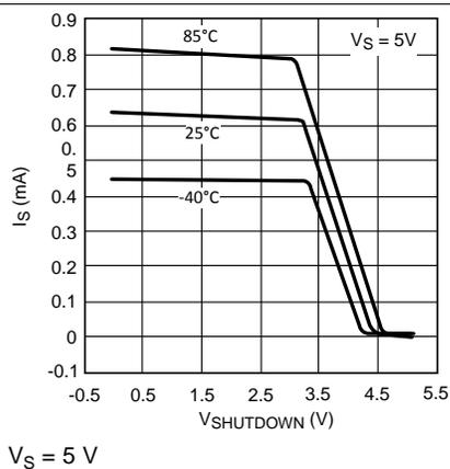
Figure 35.  $I_S$  vs.  $V_{SHUTDOWN}$  (LMH6647)
