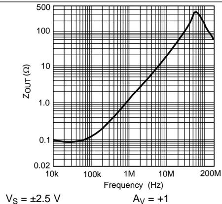
Figure 18.  $Z_{OUT}$  vs. Frequency
