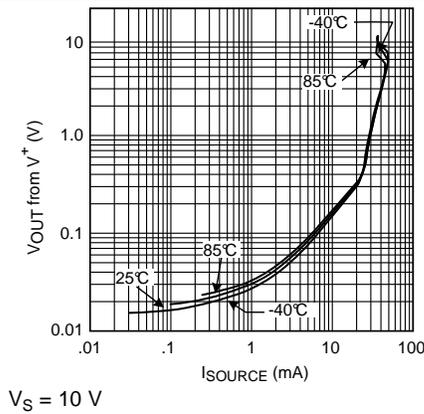
Figure 9.  $V_{OUT}$  from  $V^+$  vs.  $I_{SOURCE}$
