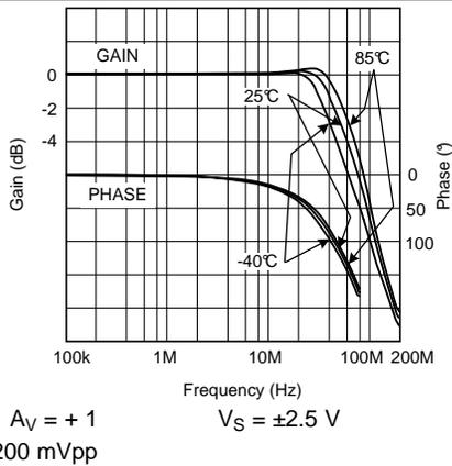
Figure 1. Closed Loop Frequency Response for Various Temperature
