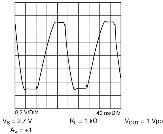
Figure 39. Large Signal Step Response
