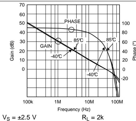
Figure 3. Open Loop Gain/Phase vs. Frequency for Various Temperature
