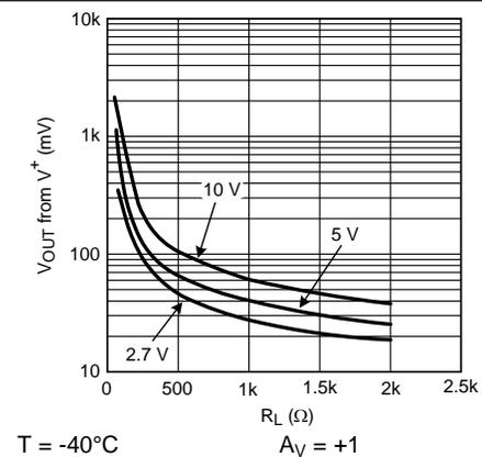
Figure 12. Output Swing from  $V^+$  vs.  $R_L$  (Tied to  $V_S/2$ )
