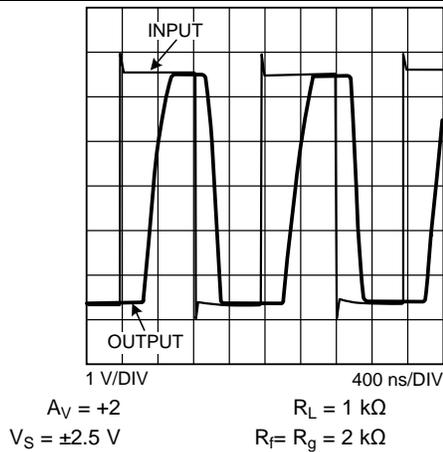
Figure 41. Output Overload Recovery
